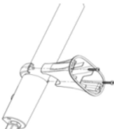
**Step 2.** Fix the tubular heater on the wall or on the floor like the following image below:
