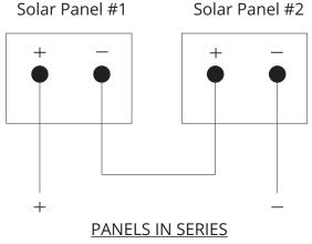
2x Single Panel Open-Circuit Voltage (VoC) 1x Single Panel Open-Circuit Voltage (VoC)
